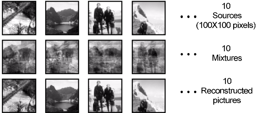
Figure 5: Four samples of a set of 10 pictures involved in the separation simulation. The mixed signals were pre-filtered by a derivative operator before the separation. The separation SIR is 20dB.
