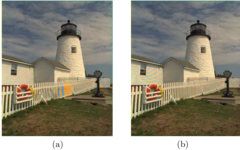
Figure 13: The output of the red and blue estimation stage (a) horizontal interpolation (b) vertical interpolation.
