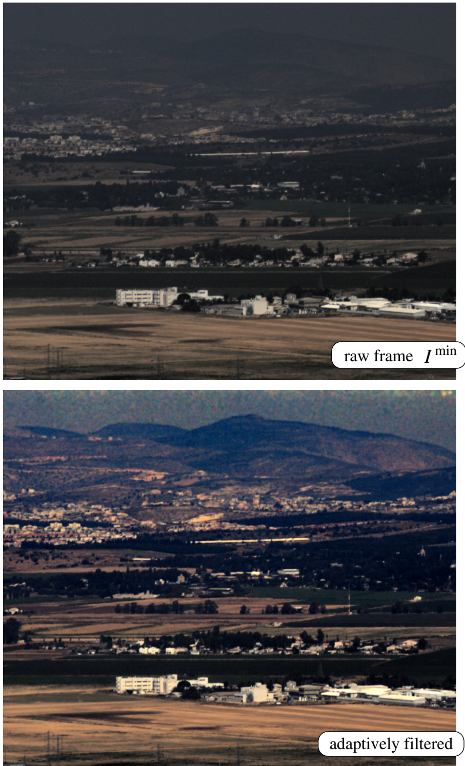
Figure 6: An additional experiment of dehazing by adaptive filtering. [Top] The raw image at the best state of the polarizer. [Bottom] Result of the algorithm.
