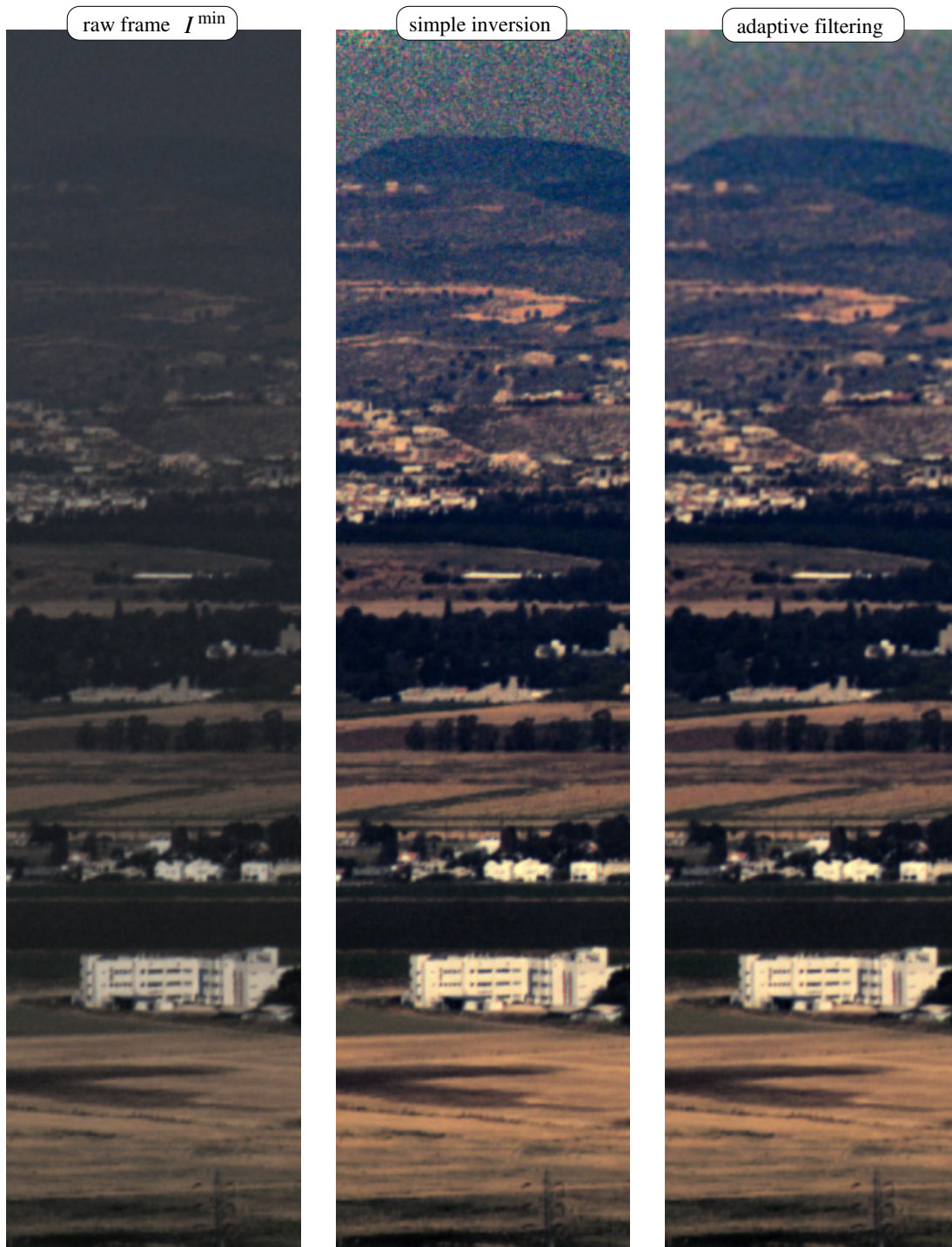
Figure 8: Zooming in on a region of the scene from Fig. 6. Dehazing by simple inversion achieves great visibility and color improvement, yet with high frequency noise in the background. Dehazing by adaptive filtering attenuates this noise, while sparing consequent blur from foreground objects.
