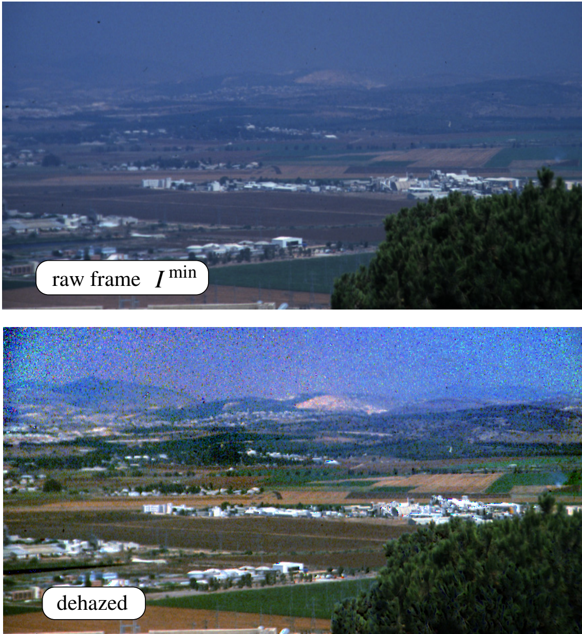
Figure 2: [Top] An image of a hazy scene, corresponding to the best state of mounted polarizer. [Bottom] Dehazed image, using the basic algorithms of [40]. While contrast is significantly improved, noise is amplified in pixels corresponding to long distances.
