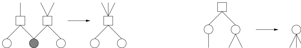
Figure 3: Graph reduction operation applied to parity-check nodes (left) and bit nodes (right).
