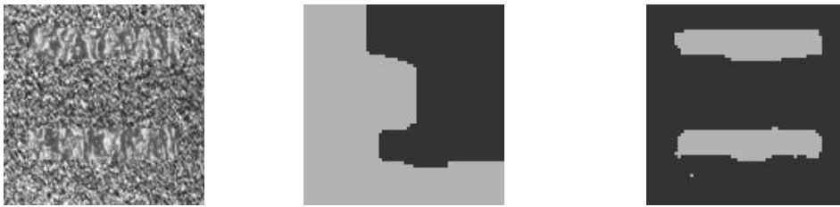
Figure 3.4: Segmentation results: (a) The original image (size 128x128), (b) Segmentation result using the wavelet transform, (c) Segmentation results using the pre-processing scheme.
