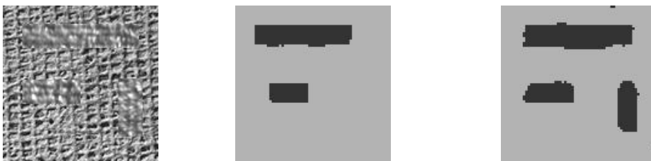
Figure 3.5: Segmentation results: (a) The original image (size 128x128), (b) Segmentation result using the wavelet transform, (c) Segmentation results using the pre-processing scheme.
