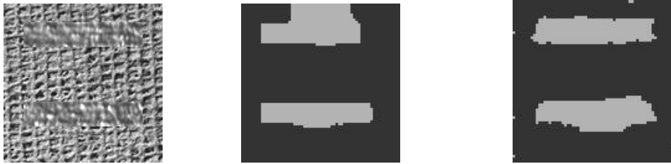
Figure 3.3: Segmentation results: (a) The original image (size 128x128), (b) Segmentation result using the wavelet transform, (c) Segmentation results using the pre-processing scheme.
