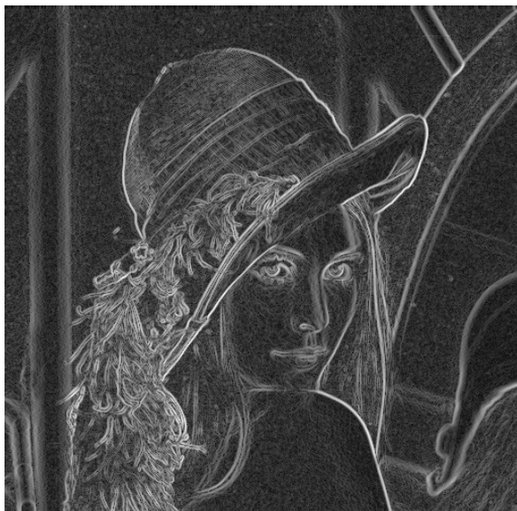
(c) Gradient values calculated by the backward difference model. Shown are the values raised by 0.4.
