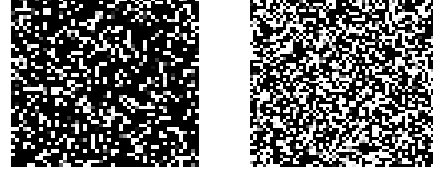
Figure 5. Multiplexing codes produced by our algorithm. [Left] N = 47, C = 12 . [Right] N = 57, C = 24 . Here, black pixels denotes w_{m,s} = 0 . White denotes w_{m,s} = 1 . The intermediate values are in gray.
