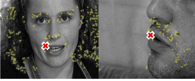
Figure 4. A frame from the speakers sequence. Out of the selected and tracked visual features [Dots], two are automatically associated to the audio [Crosses]: correctly, one per source. The audio mixture is also decoupled to two separate speakers.
