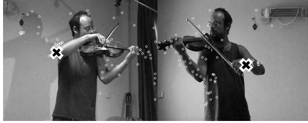
Fig. 10. A frame from the dual-violin movie. Out of the selected and tracked visual features [Dots], two are automatically associated to the audio [Crosses]: correctly, one per source.
