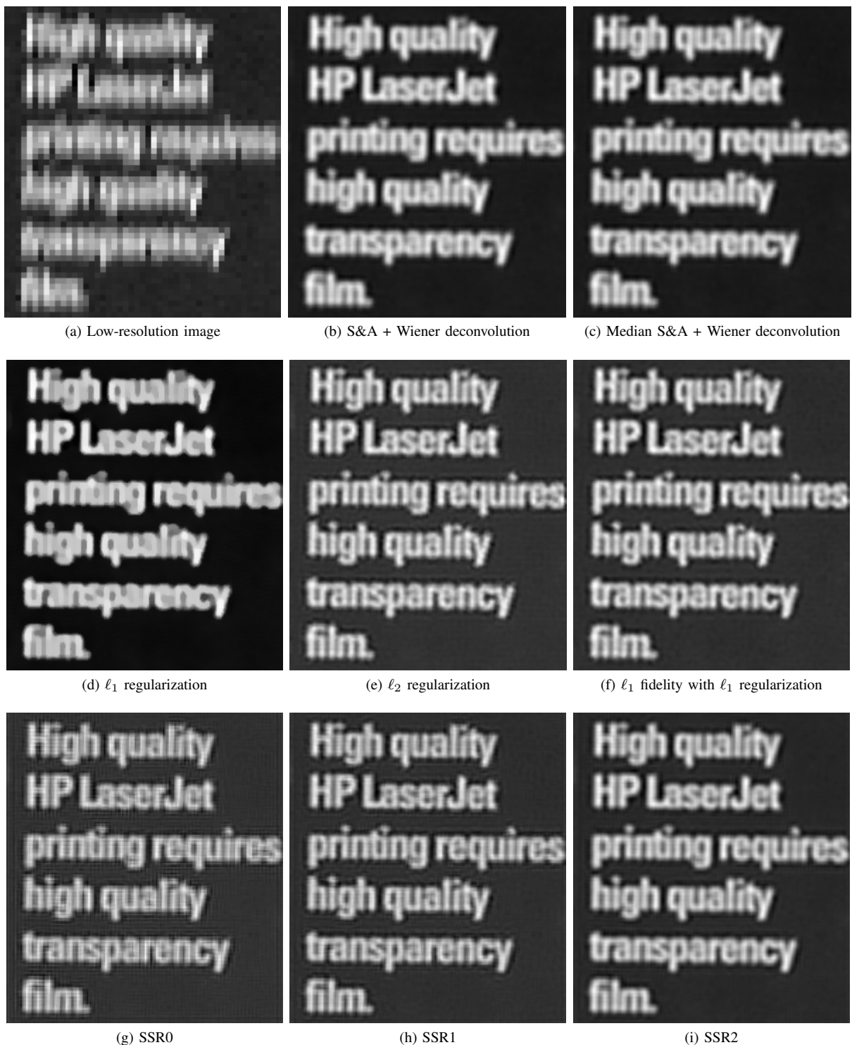
Fig. 10: Resolution enhancement by a factor of \Delta = 4 from a set of 28 images.
