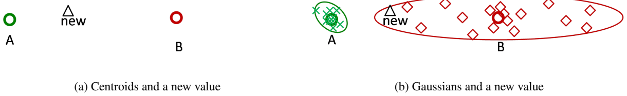
Figure 1: Associating a new value when collections are summarized (a) as centroids and (b) as Gaussians.
