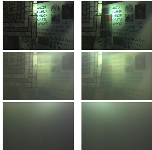
Fig. 10. (top row) stereo images in clear water, (middle row) stereo images of the same scene in turbid water made by adding milk to water, (bottom row) Backscatter at infinity for the left and the right images.
