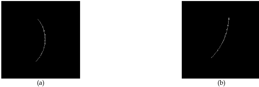
Fig. 12: Results of AGC processing of constant curvature, representing spatial adaptation along the curvature dimension. (a) is the original curve (i.e. the input to the system) and (b) is the result of (a) being processed by the AGC algorithm (i.e. the response of the model).
