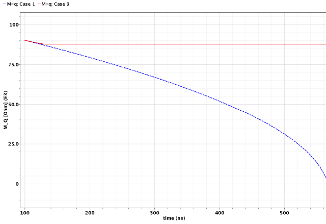
Figure 13. Memristance of q when applying an IMPLY logic gate for cases 1 (dashed line) and 3 (solid line) for a memristor with threshold model (current threshold is 7 \mu A).
