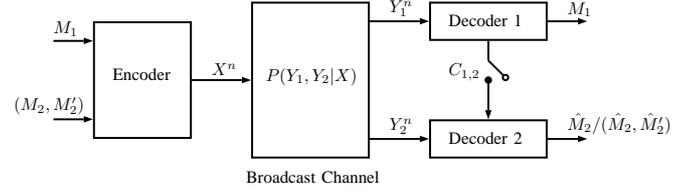
Fig. 1. Broadcast channel with unreliable cooperating decoders.
