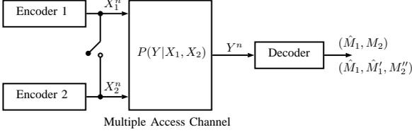
Fig. 2. MAC with unreliable cribbing encoders.
