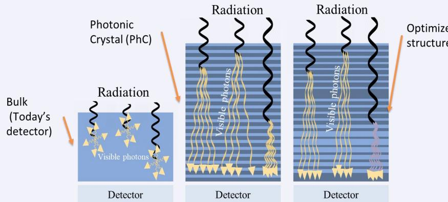
The newly designed detectors significantly outperform current detectors
